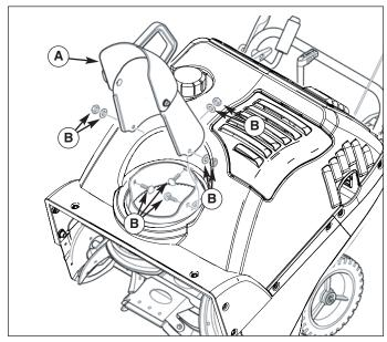
Figure 12. Chute Removal and Installation A. Chute
